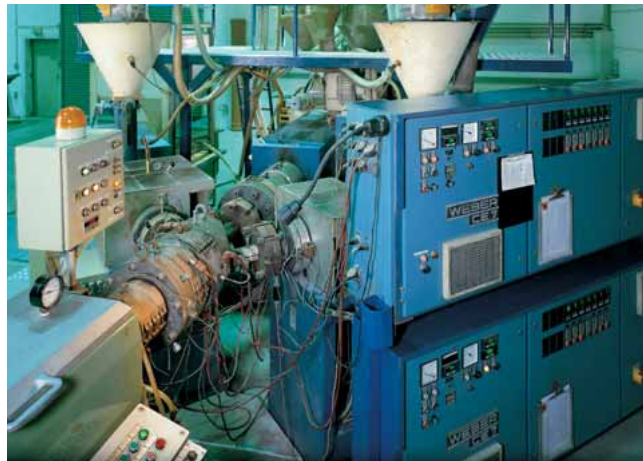
The extruder. Modern extruder plants create the prerequisites necessary for an economical, first-class pipe production.
